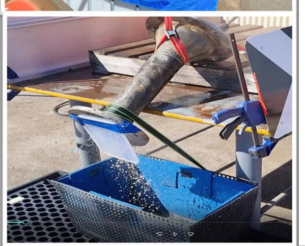
HPWC can remove corrosion scales.
